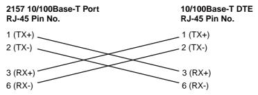
Figure 7. MDI-X switch pressed in performs 10/100Base-T crossover function
